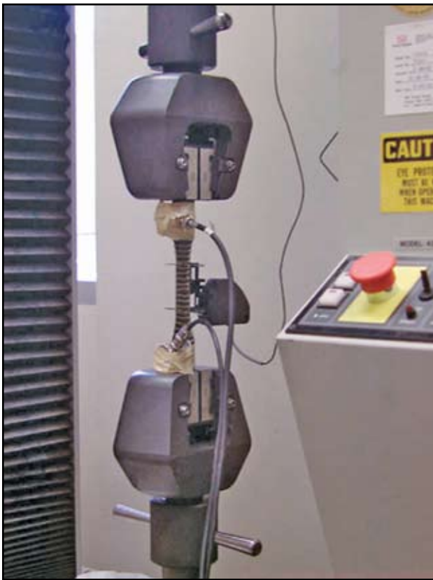
Figure 7: ASTM D3039 Testing of FRP Site Panels
