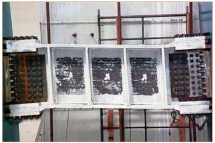
Figure 4: Full Scale Test of Shear Link Type 1 at UCSD.
