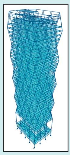
of the diagonal and horizontal elements. These nodes are one of the key design elements both structurally and architecturally. Structurally, they act as hubs for redirecting the member forces. Architecturally, they were required to not be larger than the cross dimension of the diagrid elements in order to maintain the pure appearance.
