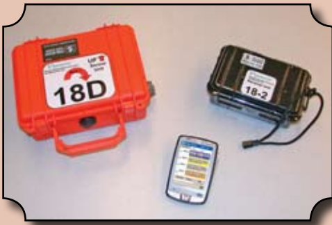
Figure 1: This monitoring system uses inclinometers and digital radio technology to detect abnormal building movement and to alert nearby personnel. It was developed by Exponent in partnership with the California Urban Search and Rescue Task Force 3.
