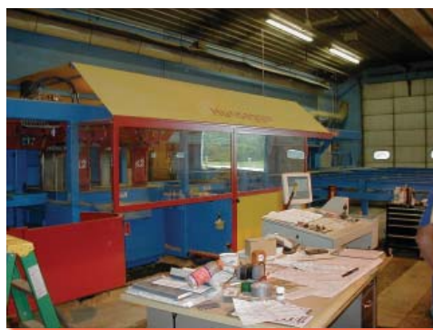
Figure 3: Computer controlled timber cutting machine
