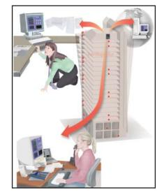
In the event of an earthquake, a predetermined structural engineer monitors incoming data to assess the building
