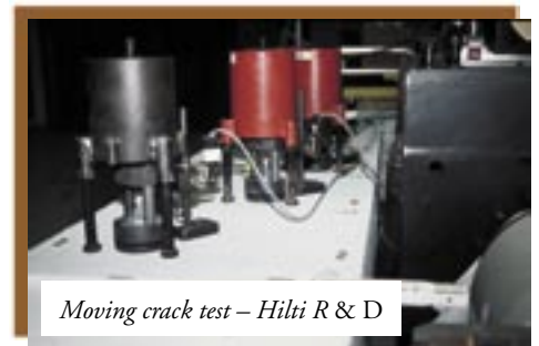
Testing in flexural cracks – Hilti R & D
