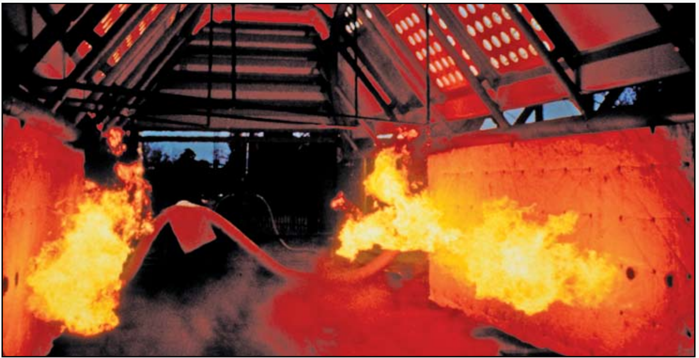
Figure 4: Fire Test of Roof Trusses for the HACTL Super Terminal 1, Chek Lap Kok Airport Hong Kong © Arup Associates
