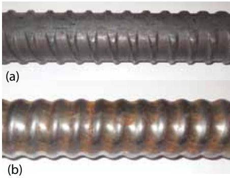
Figure 2. Typical features of threaded reinforcing bars. Continuous thread-like deformations are either (a) hot rolled or (b) cold rolled or cut into bar.
