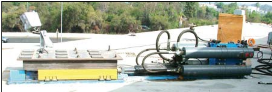
Figure 1b: Linear shaker installed on the roof of the Four Seasons Building.
