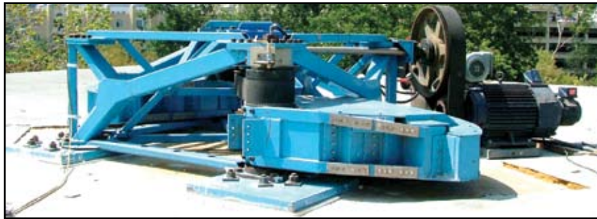
Figure 1a: Eccentric mass shaker installed on the roof of the Four Seasons Building.
