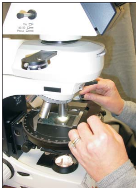
Figure 1: A thin section of concrete is shown on the stage of the petrographic microscope
