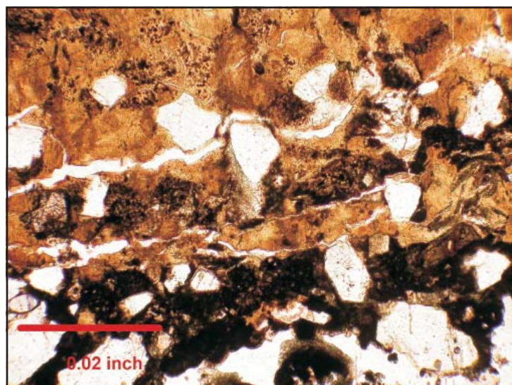
Figure 6: Exposure conditions can cause concrete to deteriorate from the outside surface inward. This concrete was placed in sulfate-rich soils in a cold moist environment.
