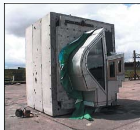
Figure 3: Arrangement for full-scale testing of the blast resistance of exterior windows in the Scottish Parliament Building. (© Arup)
