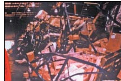
Figure 2: Storage Rack Collapse during Earthquake. Photo by Mark Pierepiekarz, courtesy of EERI.
