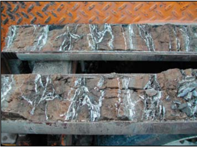
Figure 6: Example of a highly non-homogenous soil
