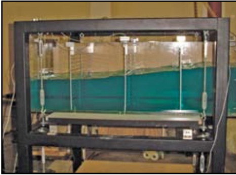
Figure 4: Single-Axis TSD Scale Model Performance Test: For fine-tuning TSD design parameters; ensuring maximum possible damping is achieved in one direction.
