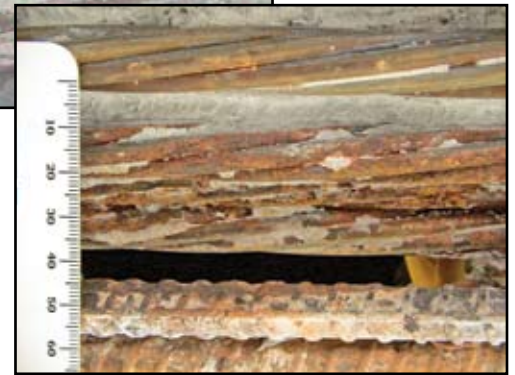
Figure 4d: Example of Level 5–6 Corrosion at Coupler
