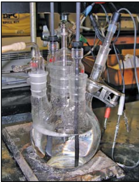
Typical electrochemical test set up for rapidly measuring corrosion rate. These methods are being developed at FPL for use on preservative treated wood.
