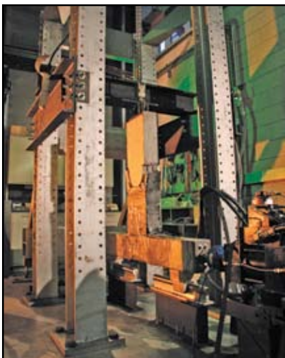
Figure 2: Specimens used in the cyclic load-displacement testing of CFRP Beam - column connection
