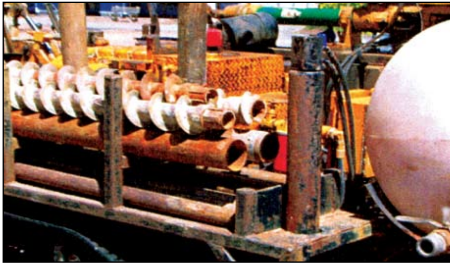
Figure 1: Hollow Stem Augers and Flush Joint Casing
