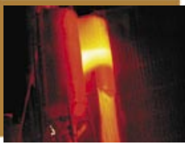
Figure 6: Thermal infrared image of a cement storage silo at a concrete batch plant. The cement in the lighter colored zone had just been placed in the silo at 6 am on this Monday morning. The cooler material below had been received the previous Friday. The cement temperature difference was sufficient to cause a 10°F concrete temperature difference between two consecutive truckloads arriving at the job site. (Source—K.Hover, Concrete International , December, 2004)
