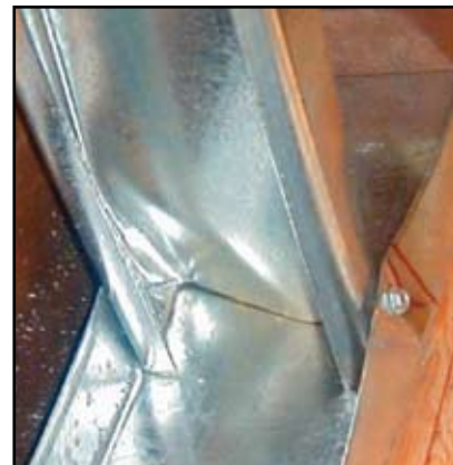
Figure 2: Stud-to-Track Assembly After Testing to Ultimate Capacity
