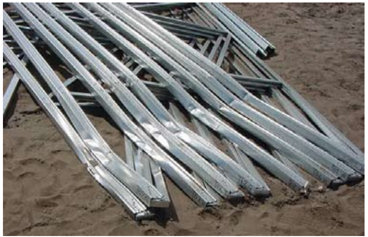
Figure 7: Field Damaged Cold-Formed Steel Trusses
