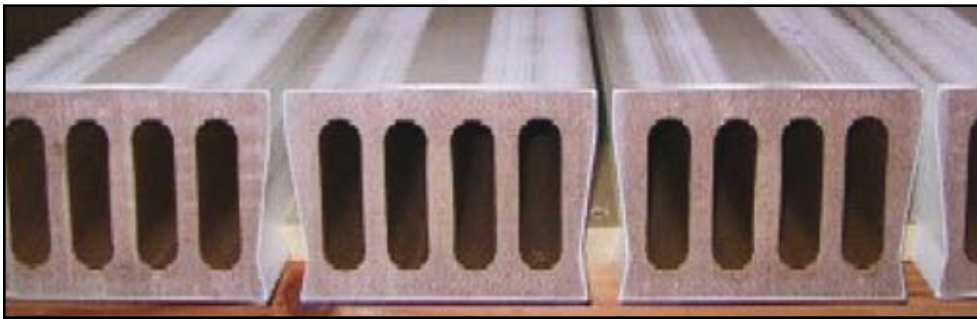
Figure 1: Capped PVC wood plastic composite deckboard prototype (4x6-inch).
