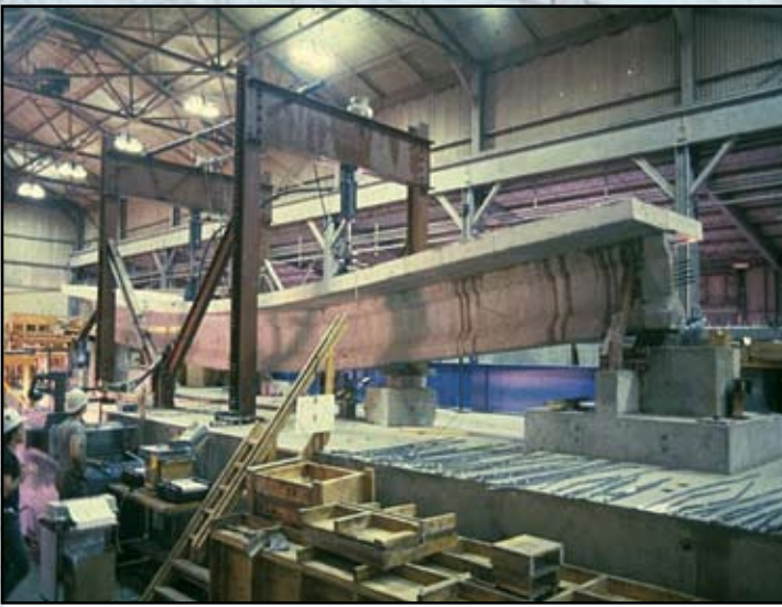
Figure 3: Fatigue Test of a full size pretensioned girder on elevated test slab.
