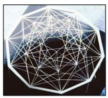
Figure 12: HB Cable Dome System.
