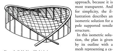
Figure 5: Cable Net of Raleigh Arena.
