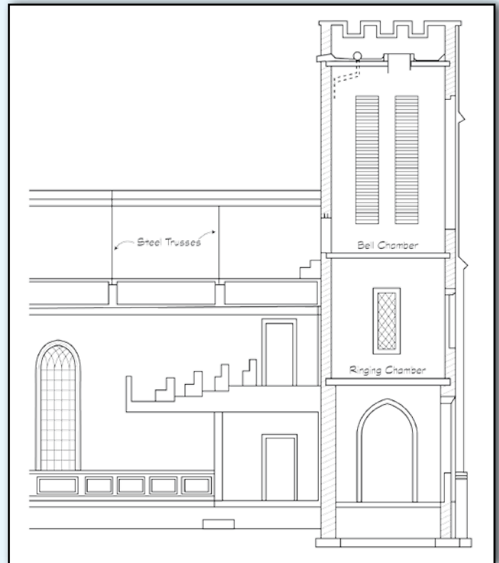
Figure 2: Tower Section from Original Plans.
