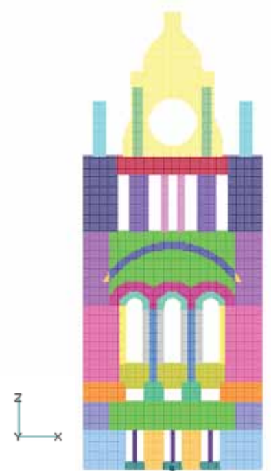
Figure 3: FE mesh of the tower masonry.
