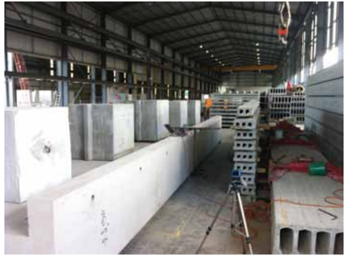
Figure 5: Full scale load test at precast factory.
