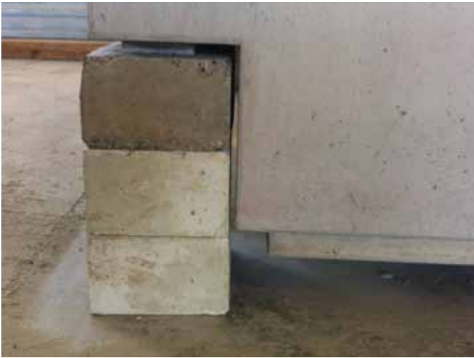
Figure 4: Support at the panel end during the full-scale test.
