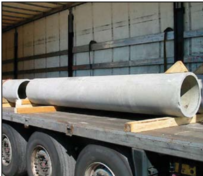
These MRC tubes were used as forms to cast load-bearing columns in the public lobby of a new high-rise building. The forms were left in place to act as blast-protection.
