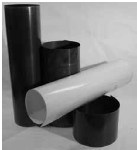
Figure 2: Carbon and glass FRP laminates.
