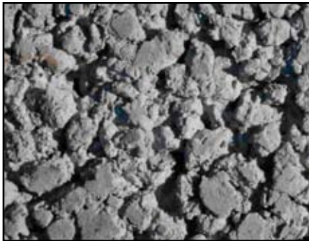
Hardened pervious concrete typically has about 20% interconnected voids.
