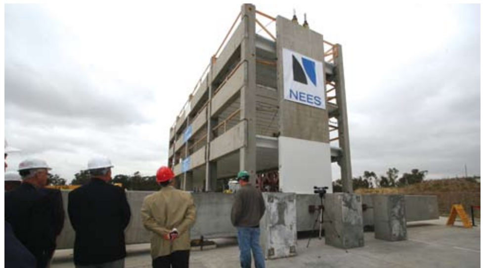
Figure 2: Half Scale Precast Structure Ready for Test on NEES@UCSD Shake Table.
