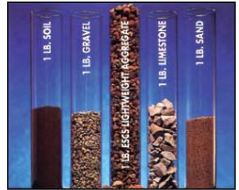
Figure 2: ESCS is half the weight of ordinary aggregates.
