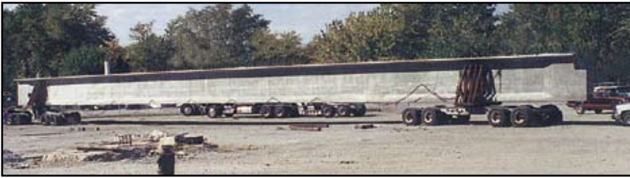
Figure 3: ESCS allows for transportation of longer precast members.
