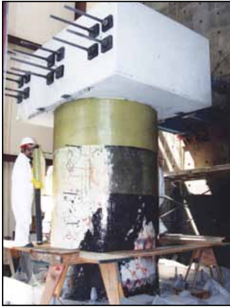
Figure 1: Wrapping of Full Scale Bridge Column at UCSD.
