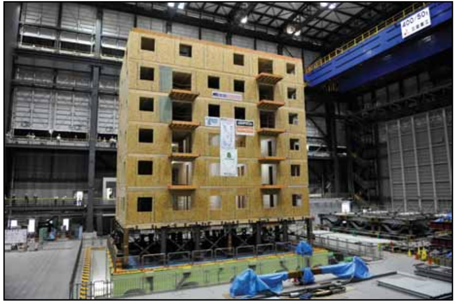
Figure 1: Completed Structure on the Shake Table.
