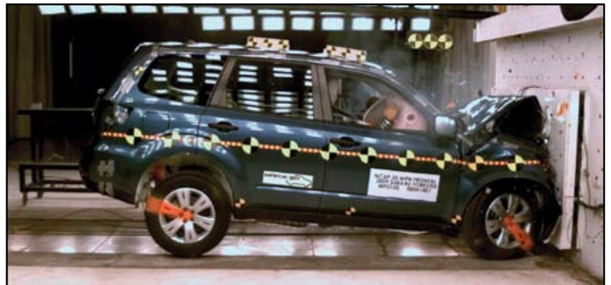
Figure 3: A car crash test on a 2009 model vehicle speeding at 35 mph against a rigid barrier. Car crush = 1 ft. 11 inches (576 mm.). Courtesy of http://nhtsa.gov .
