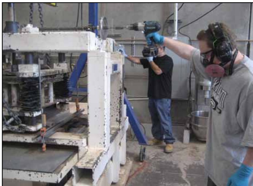
The fly ash brick manufacturing process does not use ovens, removing a major source of embodied energy and greenhouse gas emission.
