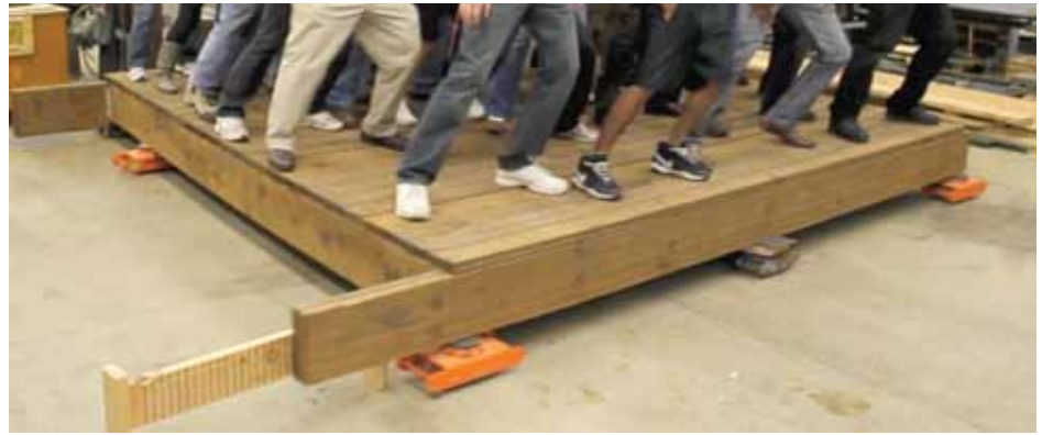
Figure 2: Cyclic loading caused by occupants swaying side-to-side in unison.
