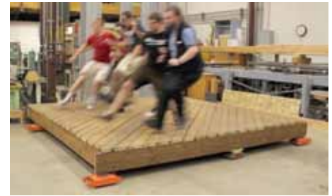
Figure 1: Impulse loading caused by occupants leaping/stopping in unison.
