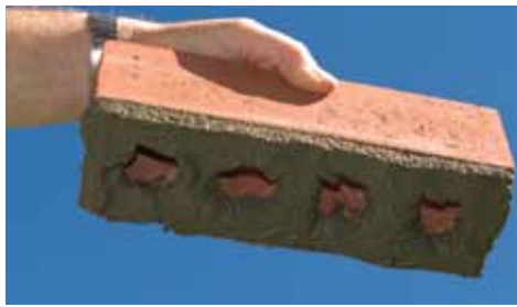
Fly Ash Brick demonstrates its mortar adhesion. In product tests, installers found it performed as well as clay brick.
