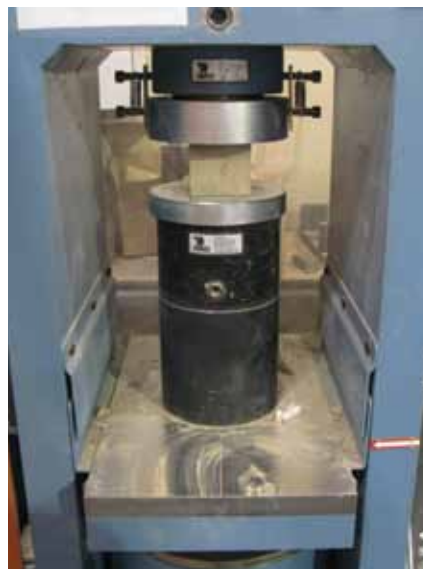
Testing compressive strength of Fly Ash Brick. When evaluating new materials, tests from existing standards can be used.
