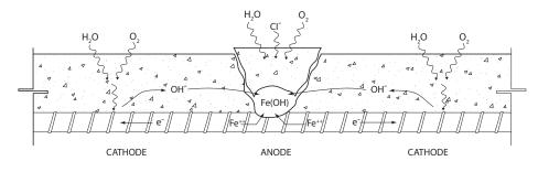
protection system is disabled. As a result, new corrosion cells rapidly occur on either side of the repair, resulting in accelerated premature failure of the surrounding concrete.
