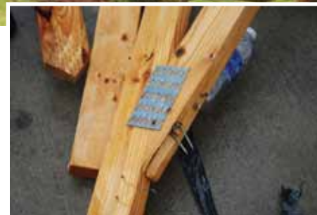
Figure 1: Toe-nailed connection for truss.
