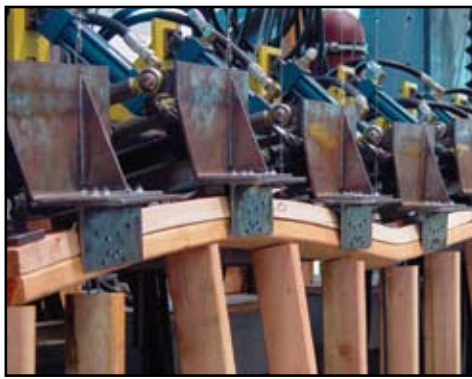
Figure 2: Obvious top plate bending in testing of rod system with 72 inch o.c. spacing at the Simpson Strong-Tie Tyrell Gilb Research Lab in Stockton, California. Ultimate load is 290 plf; using a factor of safety – 2.0, yields an allowable uplift capacity of 145 plf.
