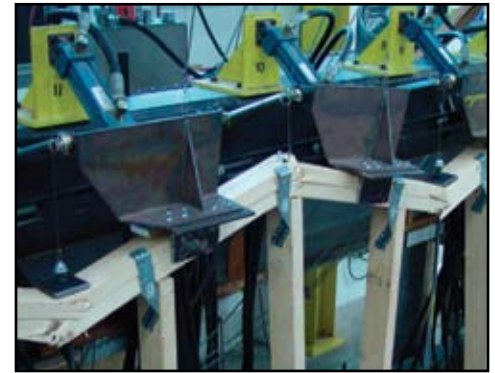
Figure 6: Simpson Strong-Tie TSP top plate to stud connectors restrain the top plate rotation, allowing the maximum load to be transferred to the rod tie-down system.
