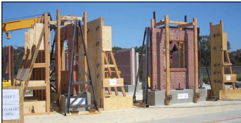
Figure 8: Testing of in- and out-of-plane wall segments on outdoor shaking table at the University of California at San Diego, September 2007.
