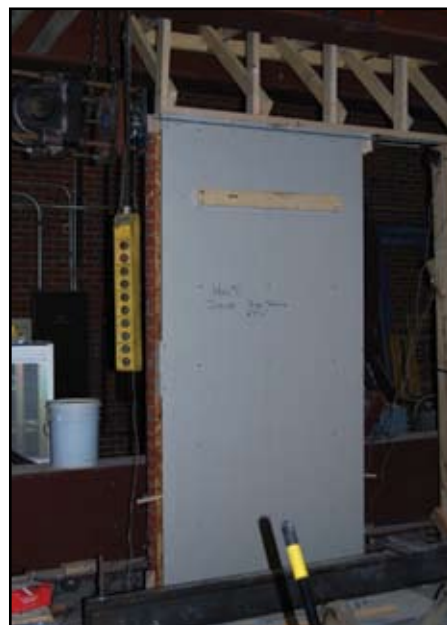
Figure 4: In-plane, quasi-static, wood-stud specimen (4-ft long) tested at North Carolina A&T State University (NCAT Wood 3).
