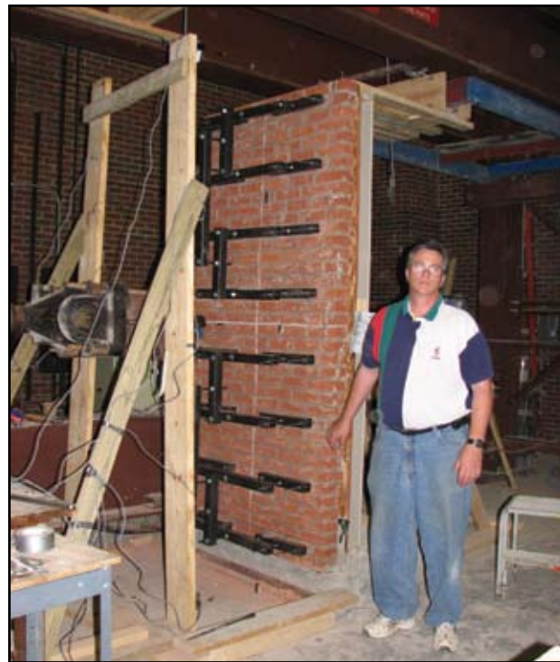
Figure 6: Typical out-of-plane, quasi-static specimen with wood-stud backing tested at North Carolina A&T State University.
