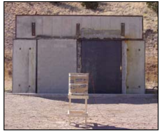
Figure 2: URM wall test specimens ready for blast test.
