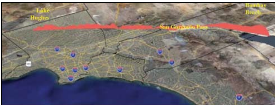
Figure 1: Scenario fault rupture. Height of the red fence indicates the fault offset at the surface. At Bombay Beach, where the fault last ruptured in 1680, the surface slip is 13 meters (40 feet).
