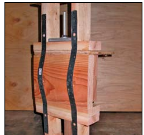
Figure 5: Top Floor Strap Termination. Rod Systems with straps spanning floors are not compatible. Demonstration shows the result of 1/4" floor shrinkage.
