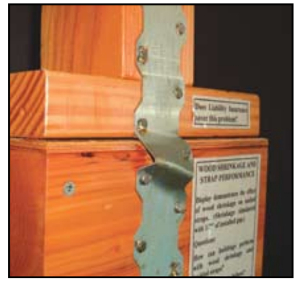
Figure 1: Typical buckled strap installation.
