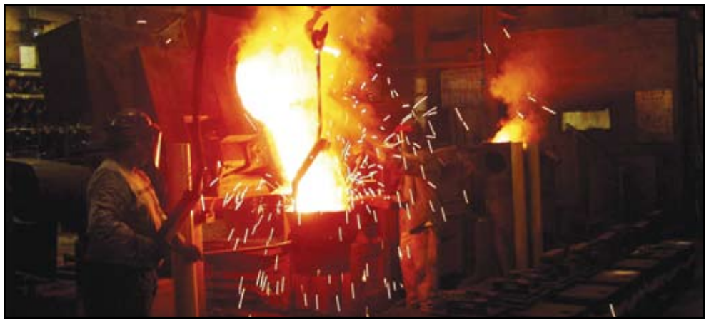
Tapping the furnace.
