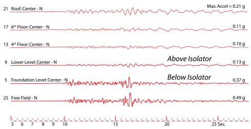
Figure 1: Strong motion records from a 7-story base-isolated hospital in Los Angeles (upper left). Accelerometers are mounted above and below the isolators (upper right). The accelerations recorded in the 1994 Northridge earthquake (lower) clearly show reduction above the isolators relative to the motion at the foundation and in a parking lot nearby.
