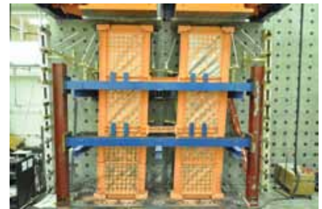
Figure 4. Coupled SPSW test at the University of Illinois. Courtesy of Daniel Borello.
