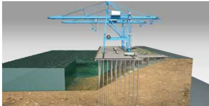
Section of wharf showing the dramatic variation in pile lengths.
