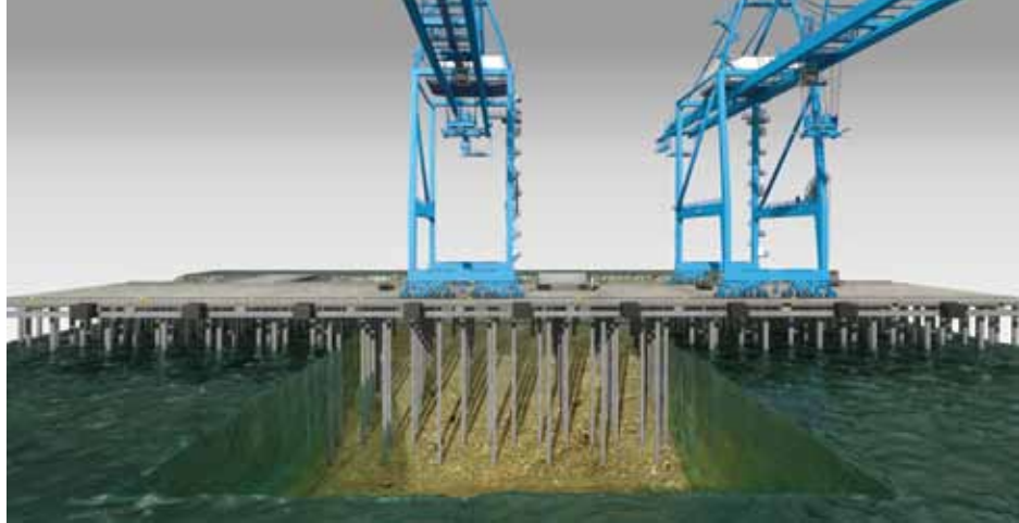
Elevation of wharf showing pile slenderness.
